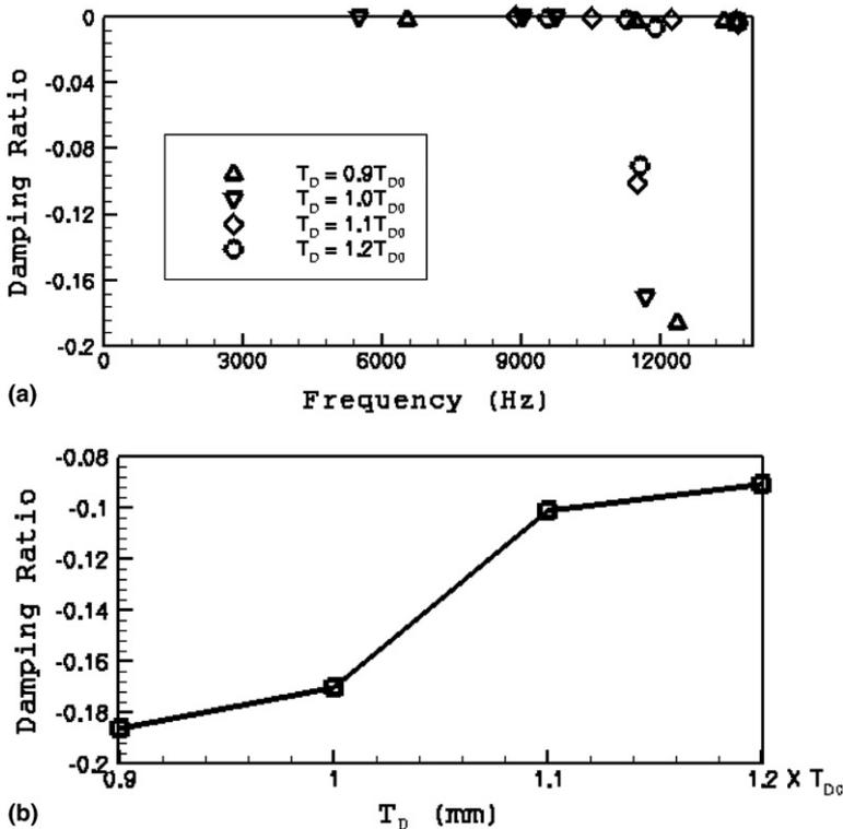
Fig. 7. (a) Variation of the damping ratio with frequency for different disc thicknesses; (b) variation of the damping ratio with thickness of the disc at frequency 12 kHz.
