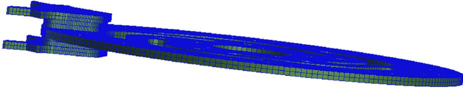
Fig. 1. Geometry and finite element mesh of the simplified disc brake system.
