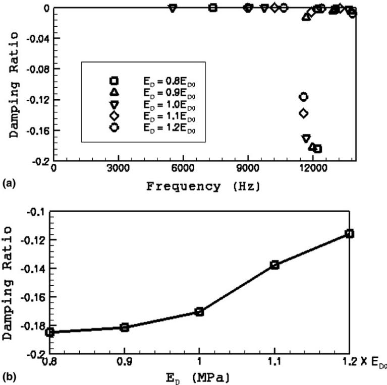
Fig. 6. (a) Variation of the damping ratio with frequency for different Young’s moduli of the disc; (b) variation of the damping ratio with Young’s moduli of the disc at frequency 12 kHz.
