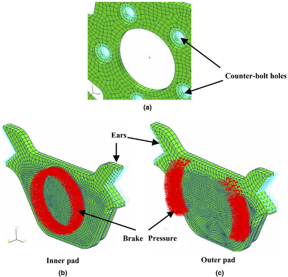
Fig. 2. Constraints and loadings of the disc brake system.
